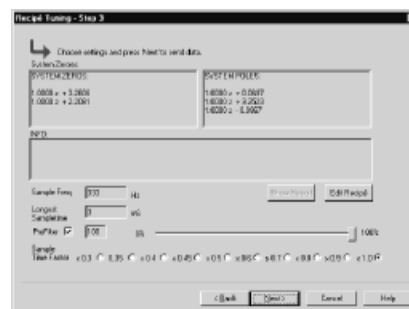
A screen display gives a super user information about the mathematical model of the system so that he can perform adjustments.
