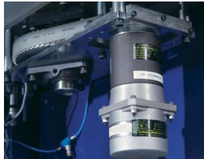
Turntable driven by step motor and gear.
